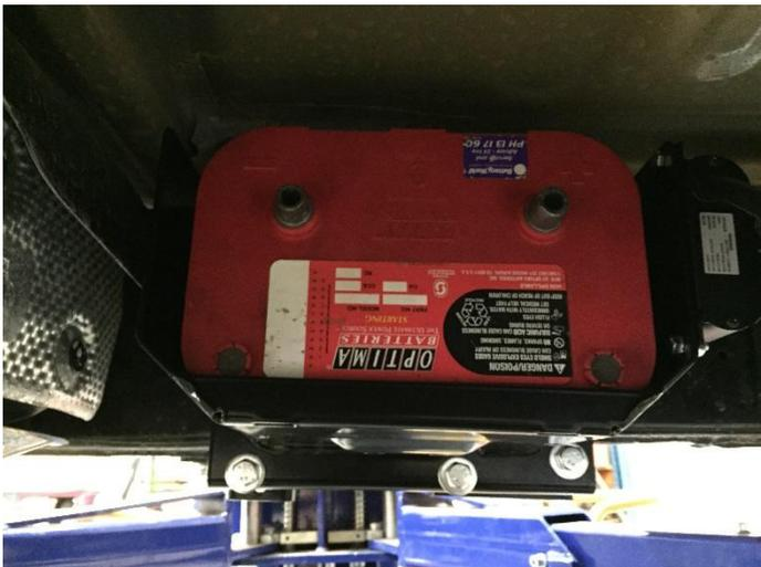
14. Fit the Battery (Optima D34 or equivalent) into Battery Tray. If a BCDC is being fitted, install the wiring as per detailed on pages 8-10.
