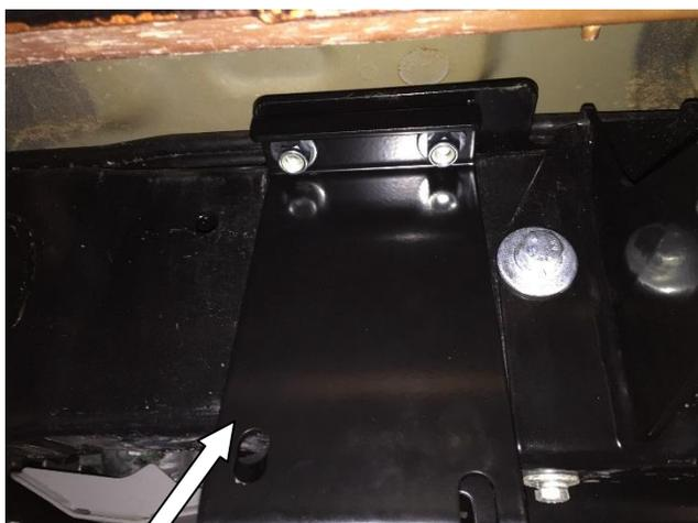
7. Ensure mounting holes (of the Battery Tray) are visible on the outboard side of the chassis. Fit Clamp Chassis Large onto the Battery Tray using 2X Bolt M10 x 1.5 x 30, 4X Washer Flat M10 x 25 x 2 and 2X Nut Nyloc M10 x 1.5. Tighten to specified torque.
